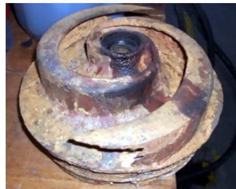
Fig. 6 Corroded mining pumping equipment
